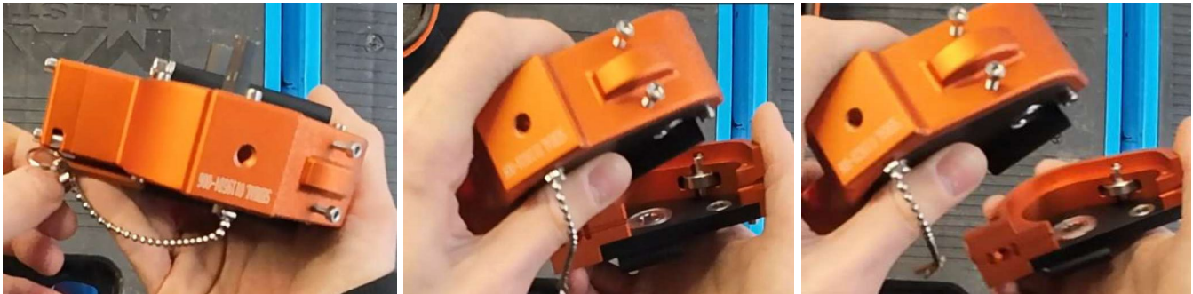
2) Removing the locking pin from its position will allow the face-plate, along with the inner wheels, to be removed from the body of the DropDrive..
